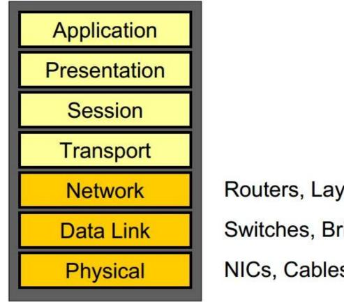
Routers, Layer 3 switches Switches, Bridges NICs, Cables, Hubs, Repeaters
