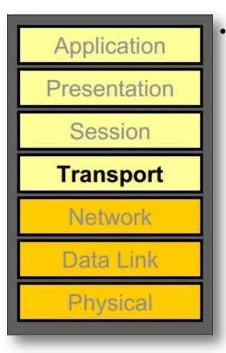
This layer provides transparent transfer of data between end systems, or hosts, and is responsible for end-to-end error recovery and flow control. It ensures complete data transfer.
