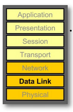
At this layer, data packets are encoded and decoded into bits. It furnishes transmission protocol knowledge and management and handles errors in the physical layer, flowcontrol and frame synchronization.
