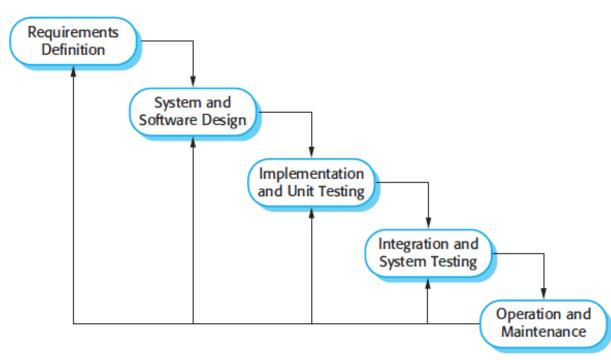
The waterfall model is a sequential design process, used in software/system development processes, in which progress is seen as flowing steadily downwards (like a waterfall) through the phases of it
